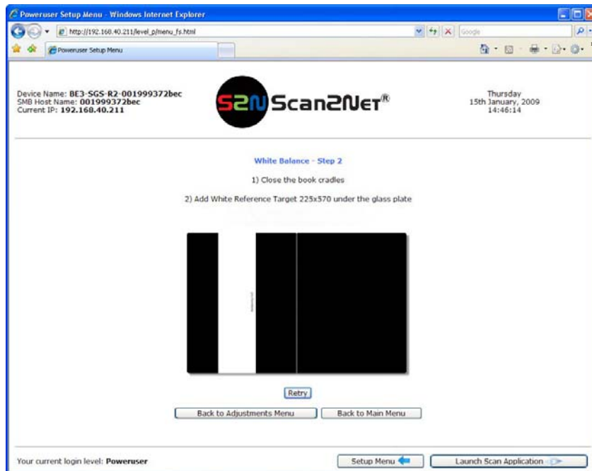
Picture 65: White Balance screen, glass plate closed
