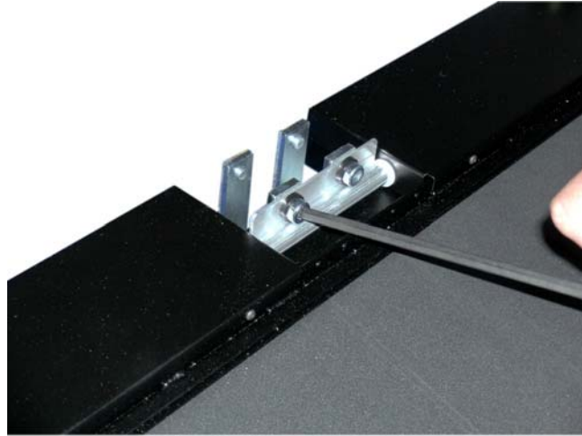
Picture 15: Removing the transport screws
