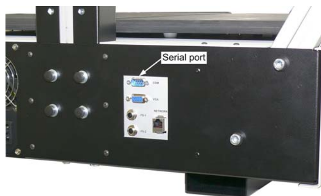
Picture 81: Connectors on rear panel
