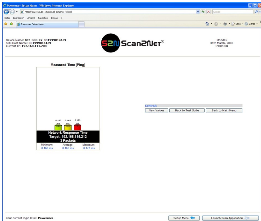
Picture 76: Network Analyzer Result screen
