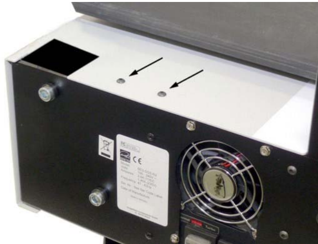
Picture 17: Remove marked screws
