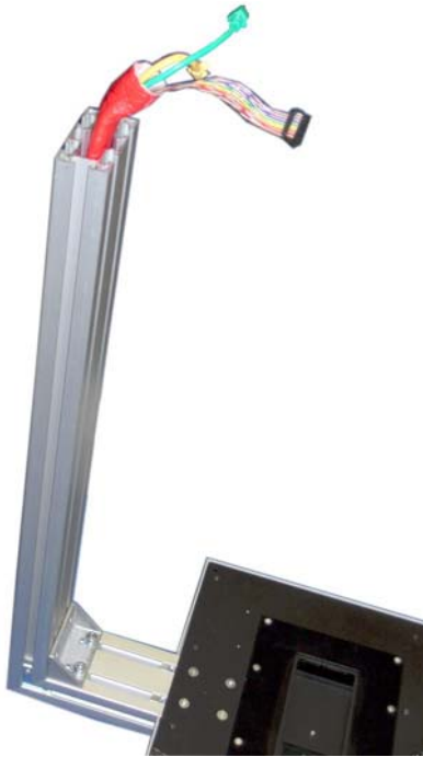
Picture 11: Camera neck assembled at camera head
