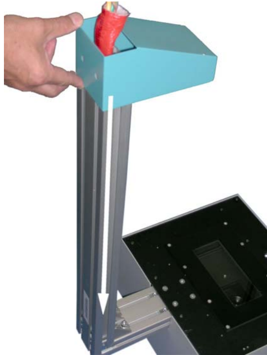
Picture 12: Placing the cover on the neck
