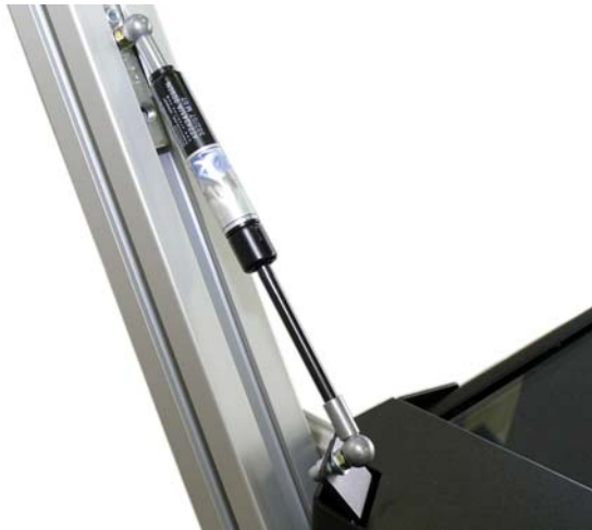
Picture 39: Gas spring completely mounted
