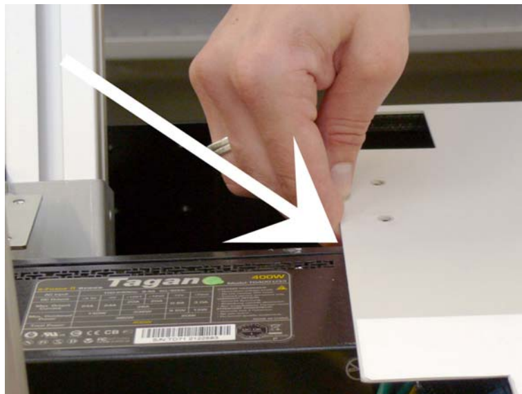
Picture 29: Body cover at edge of power supply
