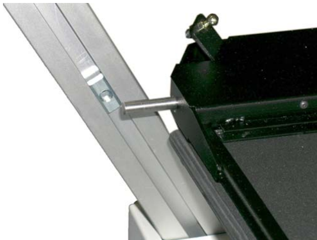
Picture 32: T-slot nut in corresponding position
