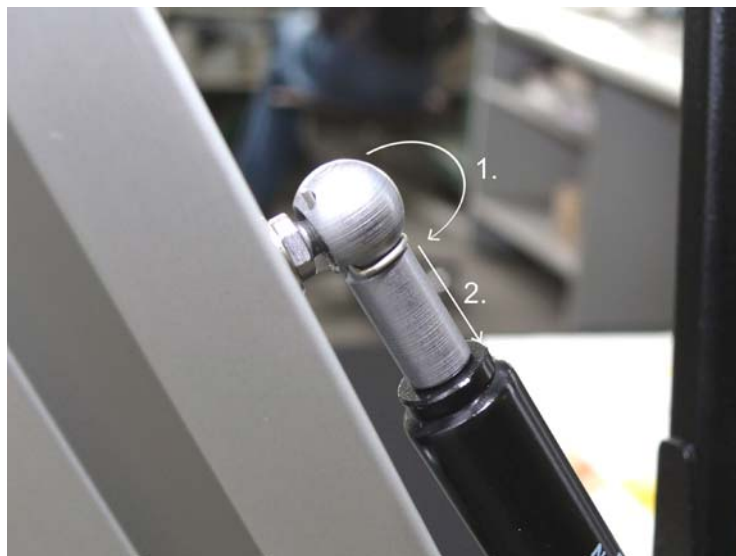
Picture 35: Removing the locking spring
