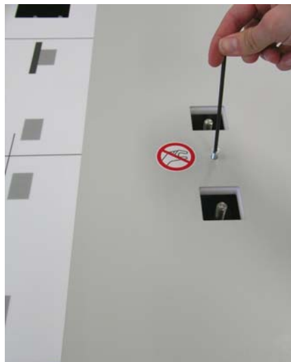
Picture 16: Removing the countersunk socket screw
