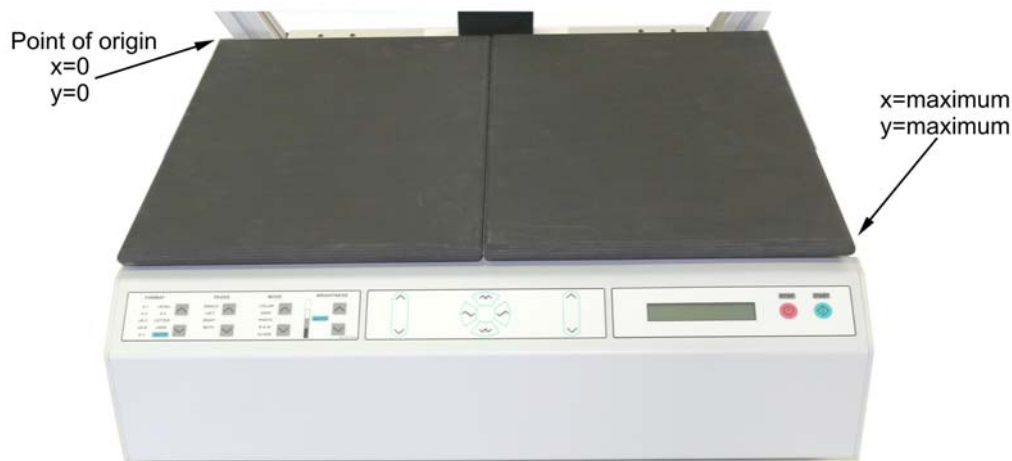
Picture 17: X- and Y Offset definition
