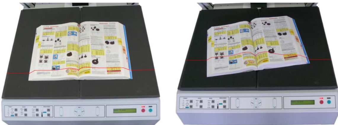
Picture 50: Correct versa incorrect placement
